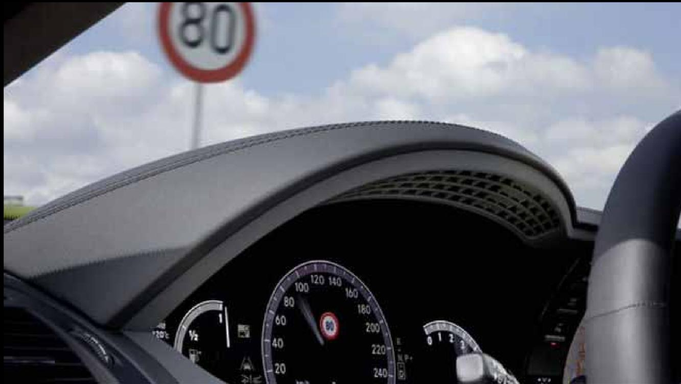
Traffic signs recognition - This is already happening in Europe, where Audi and Mercedes-Benz, among others, use front-facing cameras to identify road signs. Combining that information with the data contained in today's navigation systems, the car can replicate the speed limit right in the middle of the information cluster behind the wheel, for example.
