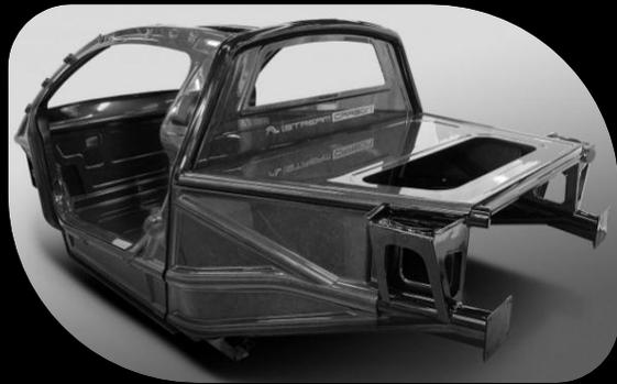
Unlike conventional carbon fiber chassis technology, iStream Carbon is a fully mechanized system with a cycle time of just 100 seconds. It utilizes two carbon skins sandwiching a honeycomb core, unlike many expensive handmade supercars which employ monolithic (single skin carbon panels).
