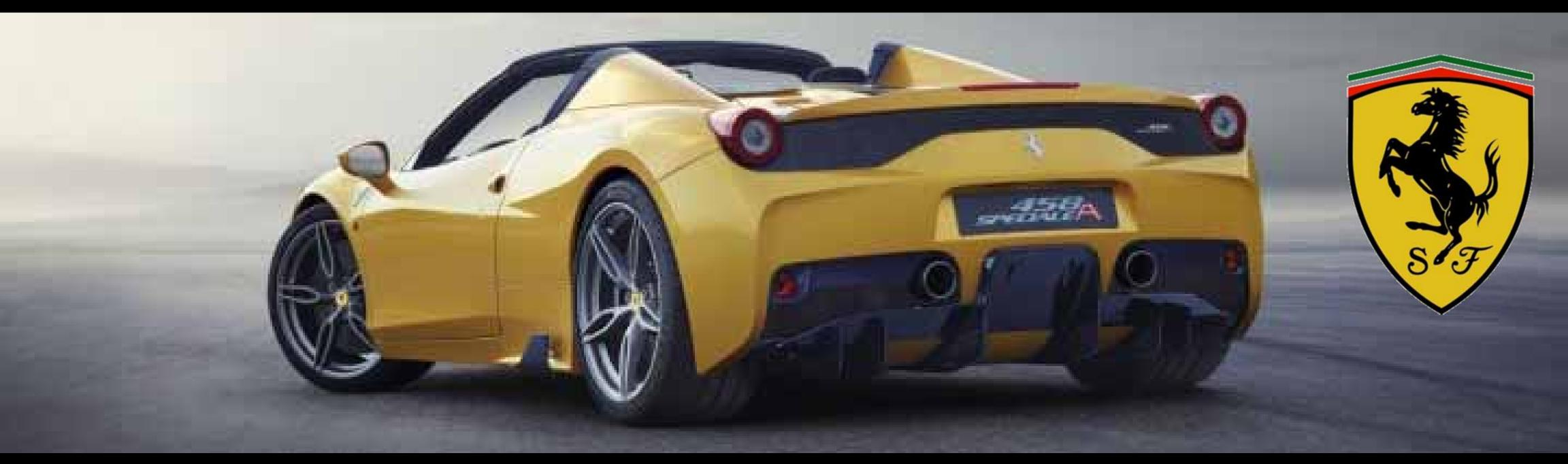
The 458 Speciale A sports the most powerful naturally-aspirated road-going V8 engine ever built by Ferrari. It has a total output of 605 cv (135 cv/l specific power output) and 540 Nm of torque at 6000 rpm, with only 275 g/km of CO2 emissions. The car sprints from 0-100 km/h in just 3.0 seconds and has a Fiorano lap time of 1'23"5, achieve also thanks to its front and rear active aerodynamics, the rigidity of a chassis that incorporates 10 aluminium alloys, and Side Slip Angle Control (SSC).
