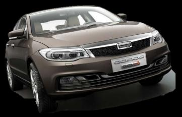
The face of the GQ3 sets the template for the Qoros model family, with wide headlamp units extending into the flanks of the car, framing the central upper grille at the same height. Horizontal LED bars feature at the upper edge of the headlights and in the distinctive rear light clusters.
