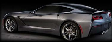
The body panels make extensive use of lightweight materials: carbon fiber for the hood and removable roof panel; composite for the fenders, doors and rear quarter panels; carbon-nano composite for the underbody panels
