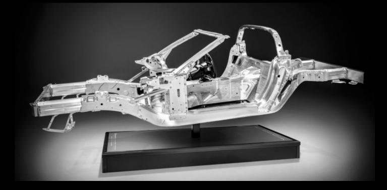
The new Corvette is based on a new aluminum frame structure which includes two main rails -each divided into five segments – with extrusions at each end, a center main rail section and hollow-cast nodes at the suspension interface points.
